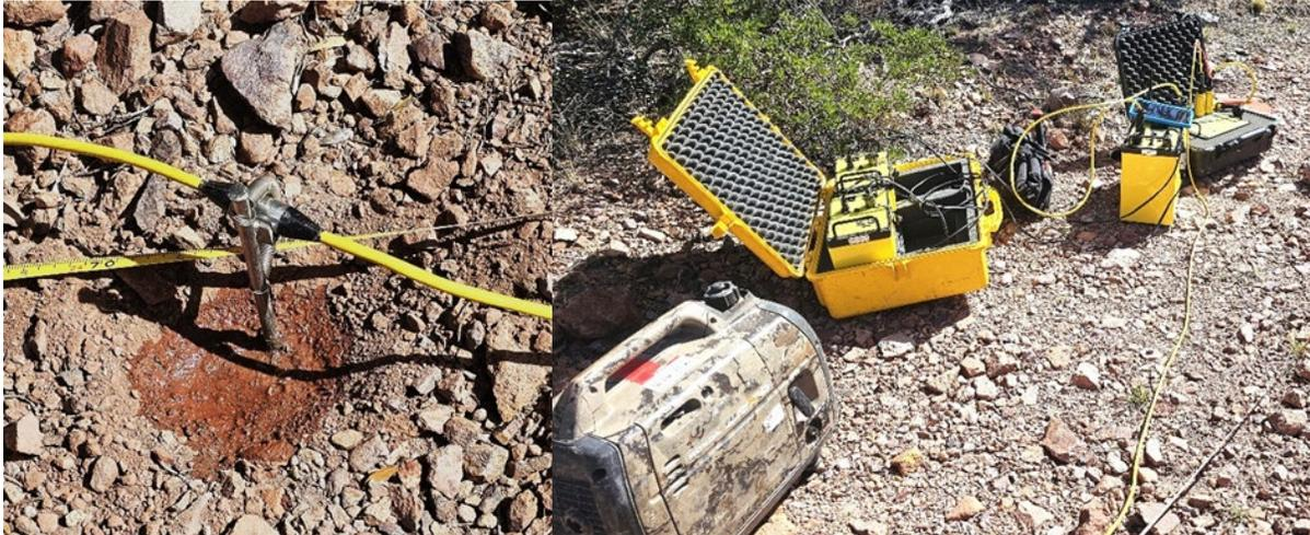
*Figure 2.1-3. Electrode array setups. Figure 2.1-4. AGI SuperSting R8 connected to a 2kW generator.*
