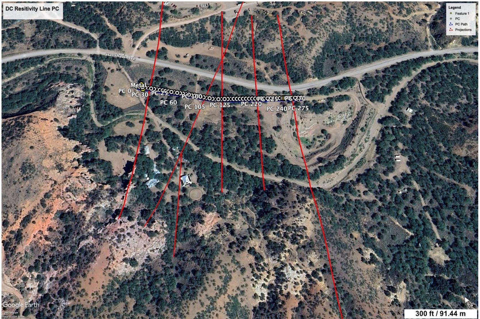
*Figure 3.2-2. Aerial image of the area around Line PC showing the linear features identified and projected onto the line.*
