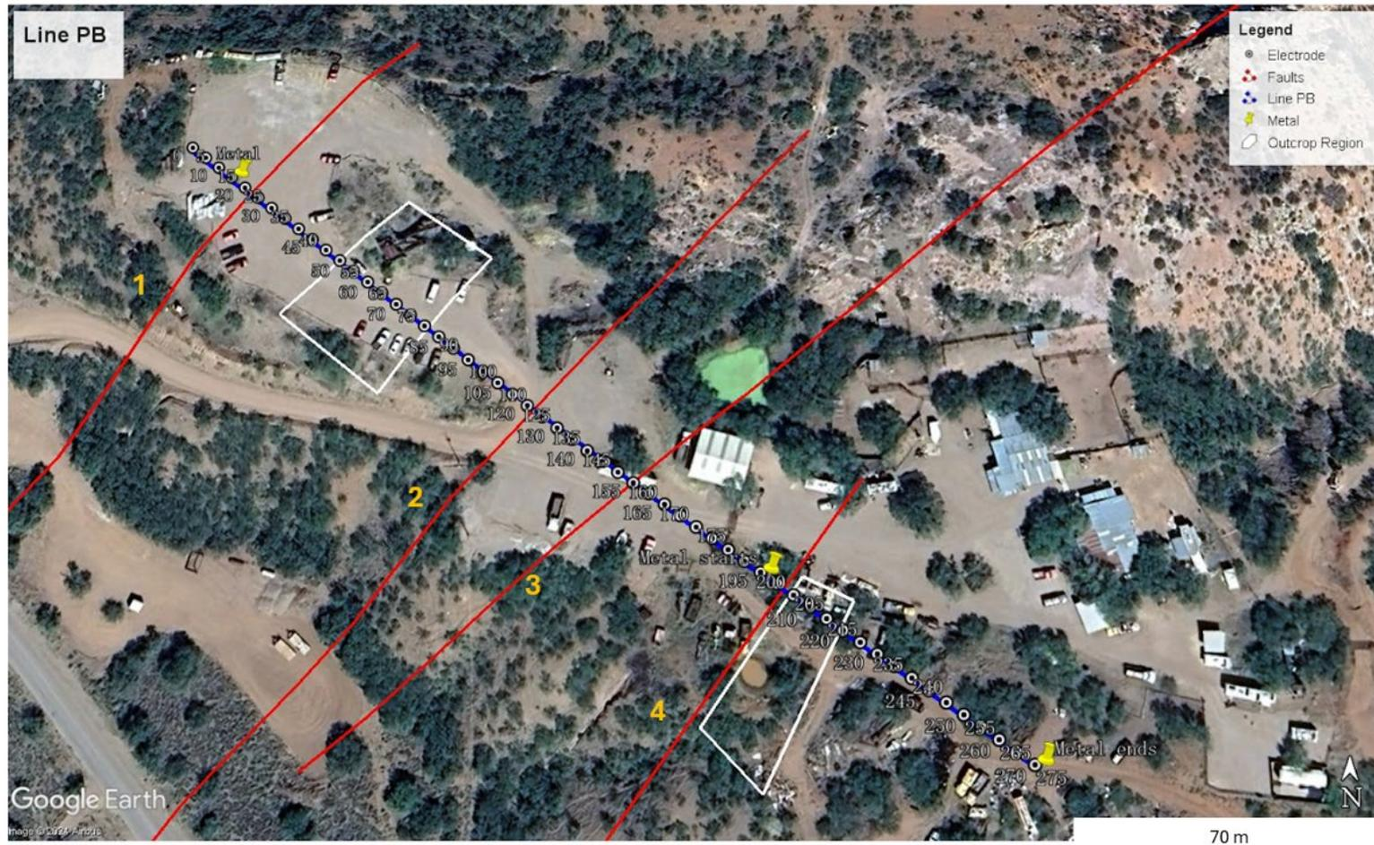
Figure 3.1-1. Map of the Line PB with potential fault lines.
